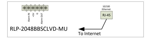
The Alarm input connections require normally closed contacts between Alarm IN and +5V for a typical setup. When the circuit opens, the Alarm Input will turn RED on the status page.
